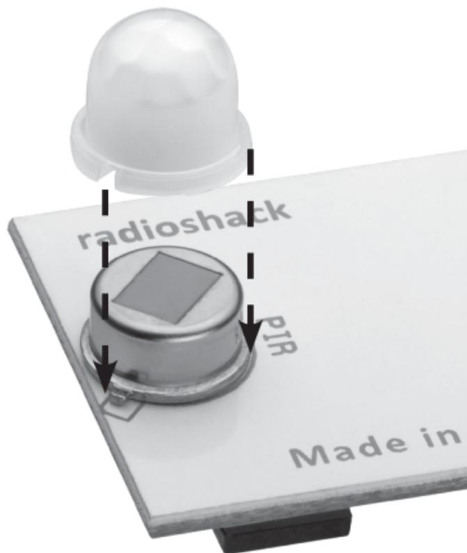
2. Connect the infrared sensor to the J11 pins on your PCB using a 3-pin cable.
