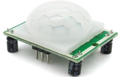
Highly integrated module popularly used for entry detection, it complies with microcontroller or DC loads.
